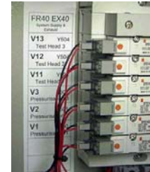
Valves rated at over 50 million cycles – An LTU6000 installation typically has to do 10 million cycles per year!
